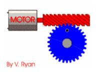
The arrangement of gears seen is called a *worm* and *wormwheel*. The worm, which in this example is brown in color, only has one tooth but it is like a screw thread. The wormwheel, colored yellow, is like a normal gear wheel or spur gear. The worm always drives the worm wheel round, it is never the opposite way round as the system tends to lock and jam.
