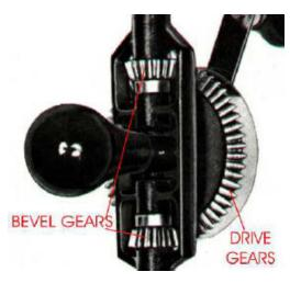
Bevel gears can be used to change the direction of drive in a gear system by 90 degrees. A good example is seen as the main mechanism for a hand drill. As the handle of the drill is turned in a vertical direction, the bevel gears change the rotation of the chuck to a horizontal rotation
