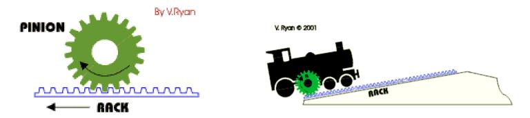
The pinion rotates and moves the rack in a straight line - another way of describing this is to say <u>'rotary motion' changes to 'linear motion'.</u>
