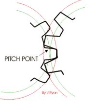
The pitch point is the point where gear teeth actually make contact with each other as they rotate.
