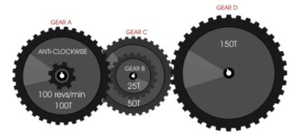
What is the revs/min at gear D and what is its direction?
