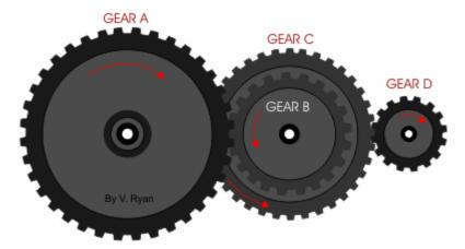
What is the output in revs/min at D and what is the direction of rotation if Gear A rotates in a clockwise direction at 30 revs/min?
