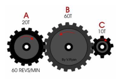
The diagram shows a gear train composed of three gears. Gear A revolves at 60 revs/min in a clockwise direction.
