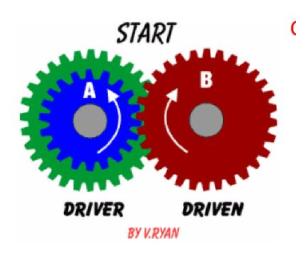
Compound gears are used in engines, workshop machines and in many other mechanical devices. In the diagram, gear 'A' is actually two gears attached to each other and they rotate around the same centre. Sometimes compound gears are used so that the final gear in a gear train rotates at the correct speed.
