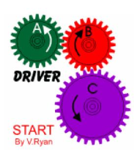
This is a good example of a 'gear train'. A gear train is usually made up of two or more gears.
