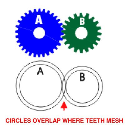
It would be very difficult to draw gears if you had to draw all the teeth every time you wanted to design a gear system. For this reason a gear can be represented by drawing two circles.
