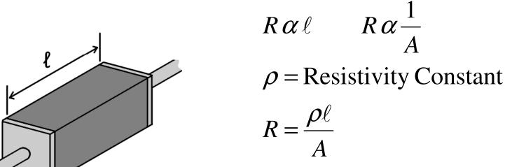
The resistance of the wire is DIRECTLY proportional to the length and inversely proportional to the area. The constant of proportionality is then defined as the RESISTIVITY, which is based on material type.
