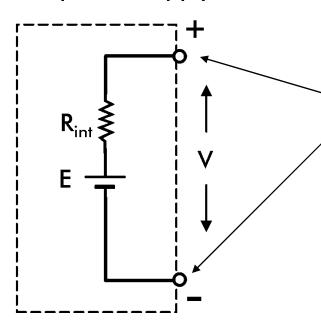
Within the schematic it will be represented as a resistor symbol next to a battery symbol and between 2 points that represent the positive and negative terminals of the battery. Many times they are labeled with letters.
