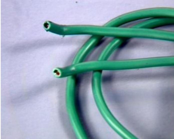
Conductor = Copper Wire
